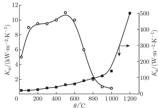
Fig. 2 Heat exchange coefficients of water and air
