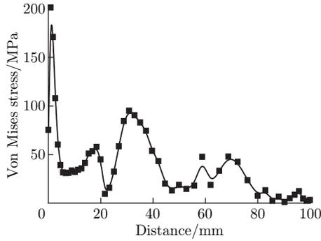
Fig. 6 Von Mises stress along the symmetric axis
