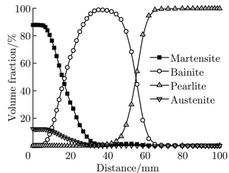
Fig. 5 Phase volume contents along the symmetric axis
