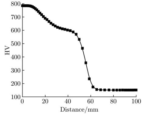
Fig. 7 Vicker hardness HV along the symmetric axis
