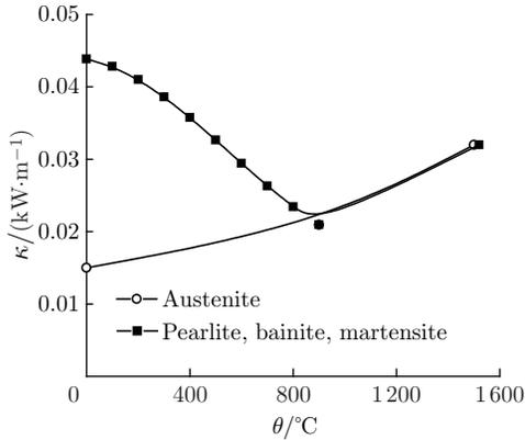
Fig. 4 Thermal conductivity values of GCr15
