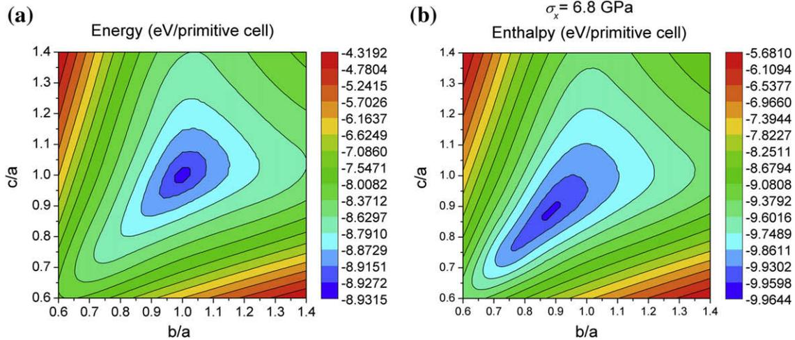
Fig. 4. Contours of: (a) energy and (b) enthalpy for uniaxial tensile stress of  $\sigma_x = 6.78$  GPa along the  $[1\ 0\ 0]$  direction based on Mishin potential.
