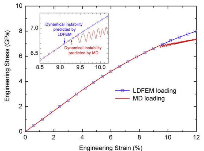
Fig. 1. Stress–strain curves of uniaxial tension along the [1 0 0] direction with LDFEM and MD simulations. The inset shows a higher magnification of the curves near the incipient instability.
