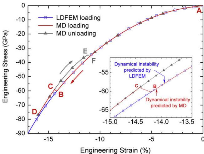
Fig. 5. Stress–strain curves of uniaxial compression along the  $[1\ 0\ 0]$  direction with LDFEM and MD simulations. The inset shows a higher magnification of the curves near the incipient instability.
