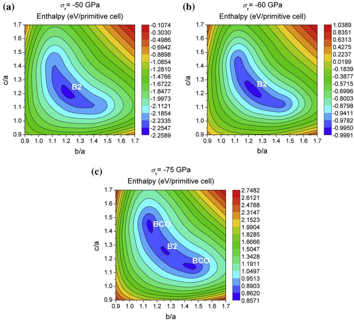
Fig. 8. Contours of enthalpy for uniaxial compression stress of: (a)  $\sigma_x = -50$  GPa, (b)  $\sigma_x = -60$  GPa, and (c)  $\sigma_x = -75$  GPa along the [1 0 0] direction based on Mishin potential. Stable or metastable structures are denoted corresponding to the minima.
