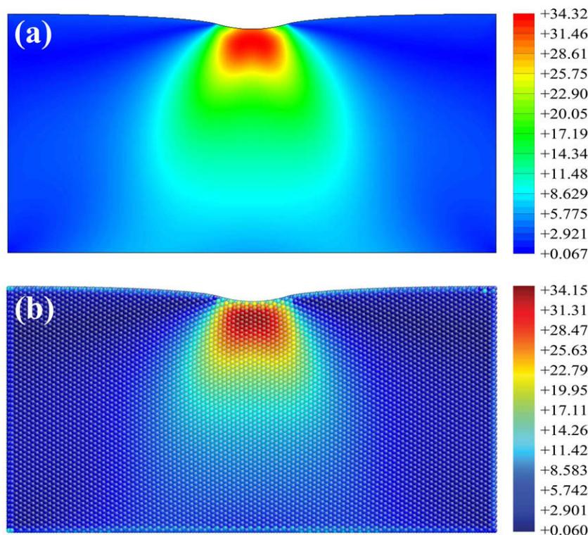
Fig. 12. Contours of von Mises stress (in GPa) at an indentation depth of 12.70 Å with: (a) LDFEM and (b) MD simulations.
