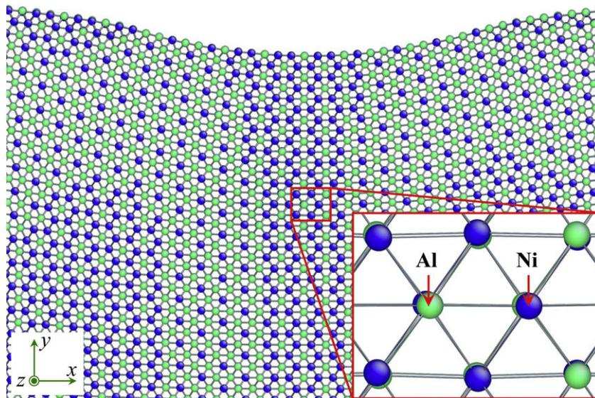
Fig. 10. Equilibrated configuration by full relaxation of the 2-D nanoindentation system at an indentation depth of  $12.71 \text{ \AA}$  with MD simulation. The inset shows a higher magnification of the region where a modulated structure appears incipiently. The coordinate system is taken as  $x = [1\ \bar{1}\ 2]$ ,  $y = [1\ 1\ 0]$  and  $z = [1\ \bar{1}\ 1]$ .
