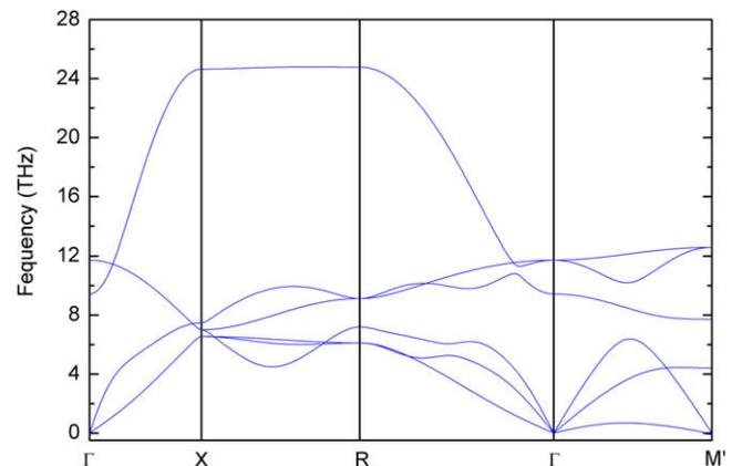
Fig. 6. Phonon spectrum along high-symmetry directions of B2-NiAl for the lattice at a strain of  $\varepsilon_x = -13.94\%$  under uniaxial compression along the  $[1\ 0\ 0]$  direction. Point  $M'$  denotes the wave vector of  $\mathbf{q}^* = [0\ 1\ 1]/2$ .
