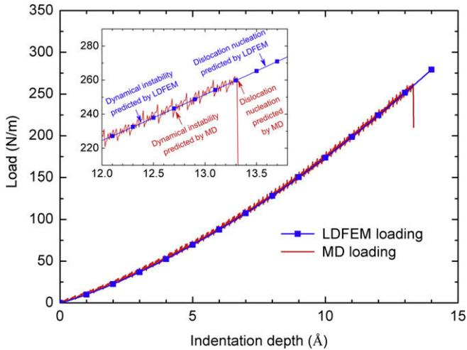
Fig. 9. Load versus indentation depth curves of the 2-D nanoindentation with LDFEM and MD simulations. The inset shows a higher magnification of the curves near the incipient instability.
