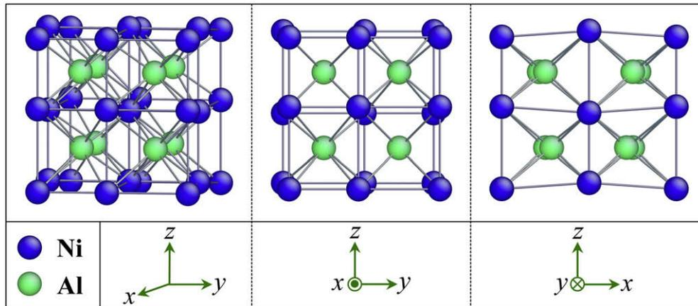
Fig. 3. Three-dimensional modulated structure of B2-NiAl at the critical strain of  $\epsilon_x = 9.28\%$  under uniaxial tension along the  $[1\ 0\ 0]$  direction with MD simulation. The modulation displacements of each atom with respect to the homogeneously strained lattice positions are enhanced to make the modulation waves visible. For all cases,  $x = [1\ 0\ 0]$ ,  $y = [0\ 1\ 0]$  and  $z = [0\ 0\ 1]$ .
