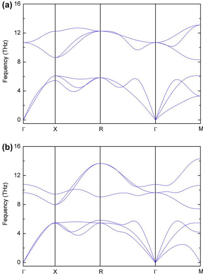
Fig. 2. Phonon spectra along high-symmetry directions of B2-NiAl for: (a) the undeformed lattice and (b) the lattice at a strain of  $\epsilon_x = 9.11\%$  under uniaxial tension along the  $[1\ 0\ 0]$  direction.
